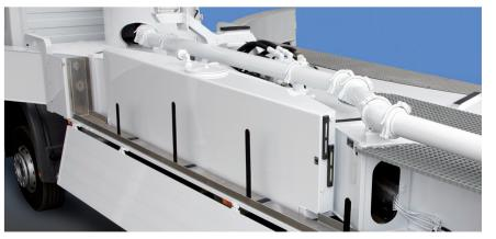
The torsion resistant frame that transfers the outrigger forces directly to the corner points provides enough space for a 600l oil tank and room for hoses and pipes.
