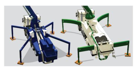
Due to the combination of front X and rear H outriggers the S 34 X can set up without the space hogging footprints of the other outrigging systems.
